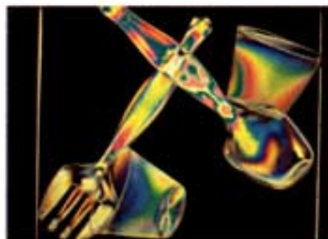
Polariscope reveals colors in white light.
