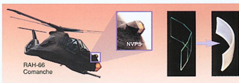
FIGURE 1. Conformal optics have aerodynamic and other advantages over conventional optics. Night Vision Pilotage System (NVPS) for a Comanche helicopter consists of a segmented window that can be replaced with a curved conformal window to reduce radar signature.
