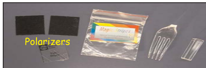
Figure 7. Contents of the Magic Stripes Theme Packet, including supplies for making a polariscope.
