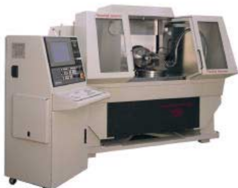
Nanotech™ 500 FG DARPA Freeform Conformal Microgrinder by Moore Nanotechnology Systems, LLC
